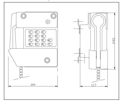
Weather-proof IP66 ACB telephone for wall mounting, aluminum light-alloy body P/N TLA346E15A
